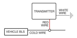
**Note:** If the vehicle has an inactive brake light switch, meaning the cold wire does not receive voltage when the key is in the tow position, connect the red wire to the blue wire on the DUO system.
